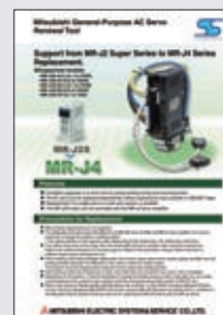
MR-J2S Renewal Tool Catalog X901307-312 This guide introduces a renewal tool for replacing MR-J2S with MR-J4. The renewal tool allows to use the existing wiring and mounting holes, making the replacement simple and fast. Mitsubishi Electric System & Service Co., Ltd.
